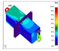
Provide (2) End plates of thickness 16 mm (5/8") with (4) 5/8" dia. bolts of grade A325 (M16 bolts of grade 8.8) using 8 mm (5/16") fillet weld on both sides and butt weld on top and bottom of plates
