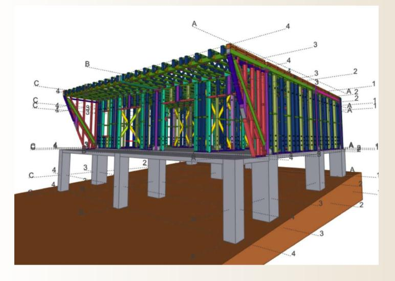
The IFC file (above) is an interactive 3D model of the building structure
